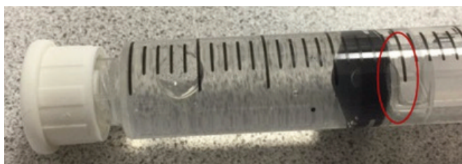
Figure 1. Medication or solutions drawn into this syringe have leaked below the black plunger (circled in red), which may pose a problem with sterility and safe handling of hazardous drugs.
